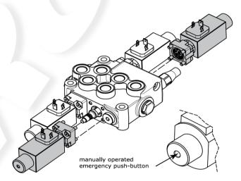
The H036 and H037 direct electric controls come as two kits each including a: spring, solenoid and adapter. The Direct electric controls use a type E special spool and a type special body.
