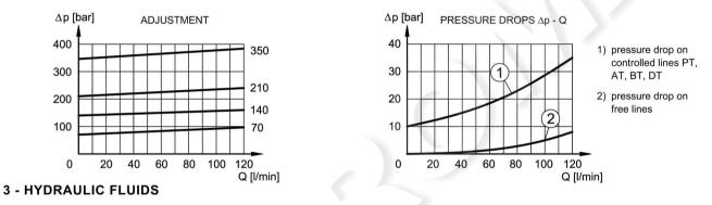
Use mineral oil-based hydraulic fluids HL or HM type, according to ISO 6743-4. For these fluids, use NBR seals (code N). For fluids HFDR type (phosphate esters) use FPM seals (code V). For the use of other kinds of fluid such as HFA, HFB, HFC, please consult our technical department. Using fluids at temperatures higher than 80 °C causes a faster degradation of the fluid and of the seals characteristics. The fluid must be preserved in its physical and chemical characteristics.
